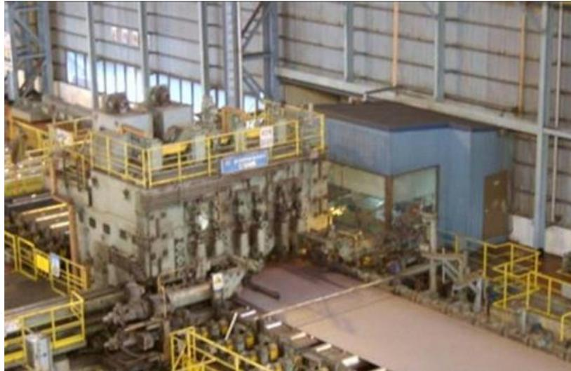
Gambar 2.10 Mesin DS (*Dividing Shear*)
