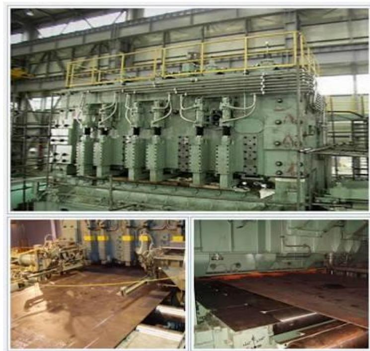
Gambar 2.8 Fasilitas Mesin *CS (Crop Shear)*
