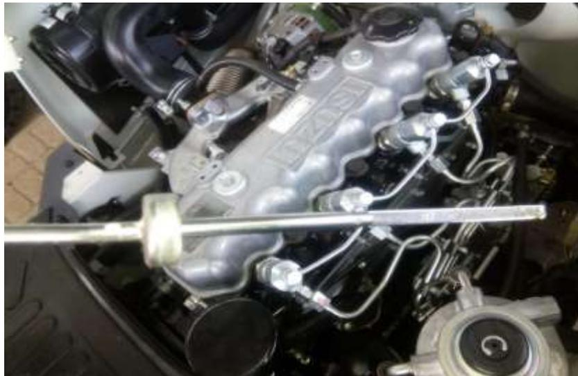
**Gambar 4.1 Level oil engine**
