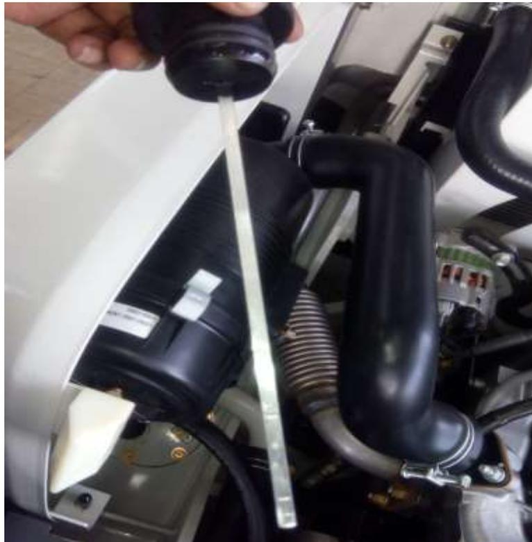
**Gambar 4.3 Level oil hydrolic**
