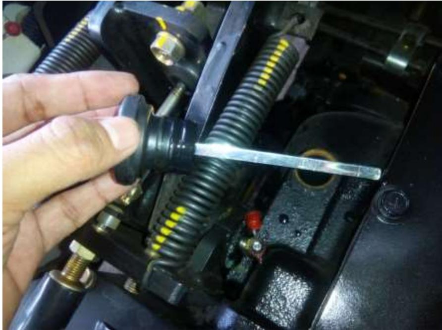
**Gambar 4.4 Level oil transmisi**
