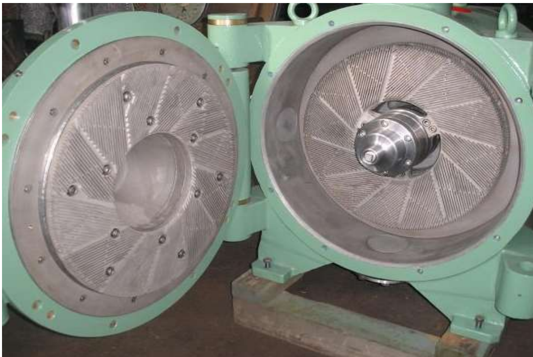
Gambar 2 Refiner Paper Machine.
