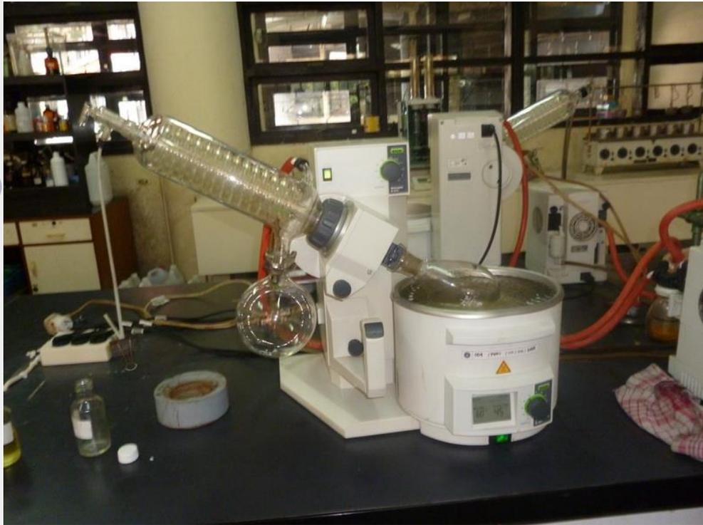
Proses evaporasi biodiesel
